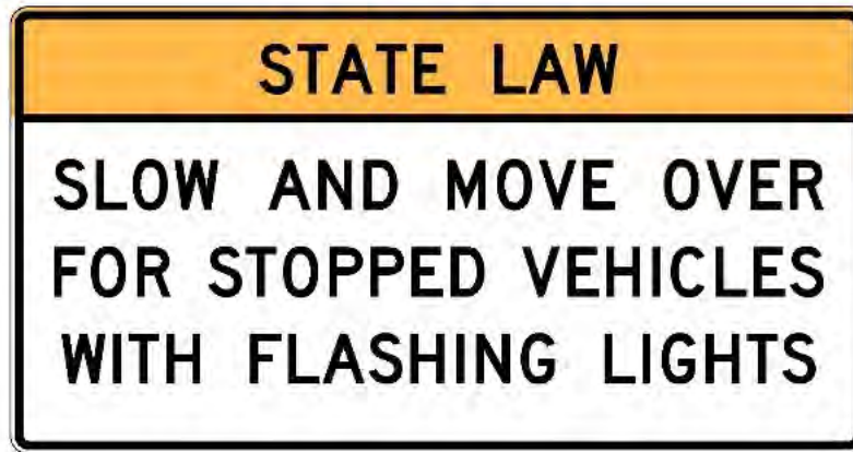
Figure 2B-33. Slow And Move Over For Stopped Vehicles With Flashing Lights Sign
