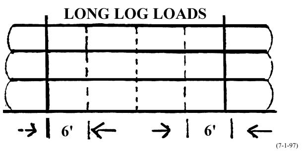
**b.** All exposed outside logs shall be secured by one (1) wrapper passing near each end of the log. See Figure 010.10-A.
