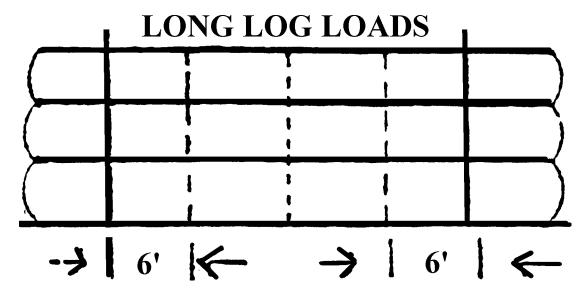
${f b.}$  All exposed outside logs shall be secured by one (1) wrapper passing near each end of the log. See Figure 010.10-A. (7-1-97)
