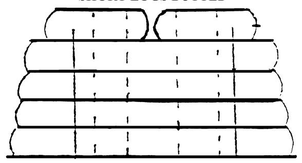
**c.** On one (1) log load where trailer bunk is equipped with cheese blocks, one (1) wrapper securing log to the trailer bunk will be sufficient. Outside wrappers on short logs shall have a minimum of six (6) feet spread.(See Figure 010.10-C.)
